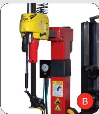
**EN** **VERTICAL POST:** Designed for extra heavy duty purposes and equipped with automatic swing arm movement and triple regulation system for easy maintenance activity. To achieve a better level of safety and accuracy, the working arm is pneumatically controlled and the horizontal arm is equipped with a double locking system and with rollers to improve the fluidity of its movement.
