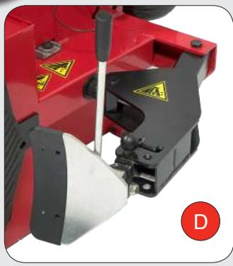
**EN** **BEAD BREAKING SYSTEM:** Bead breaker arm equipped with high efficiency double acting cylinder and with a Teco patented system which allows exactly the right position no matter the wheel diameter or width, thus improving the accuracy of bead breaking operations. Also the wheel support is adjustable in 2 different positions.
